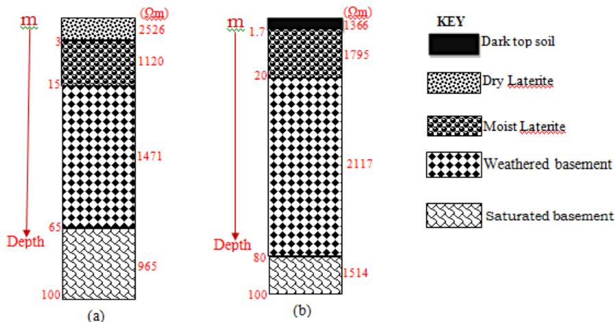
Figure 3: Geo-electric and inferred geologic sections for VES 1 and VES 2 respectively
