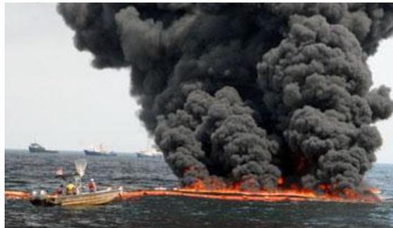
Figure 6: In situ burning of an oil slick, or part of a slick, before it reaches the coast
