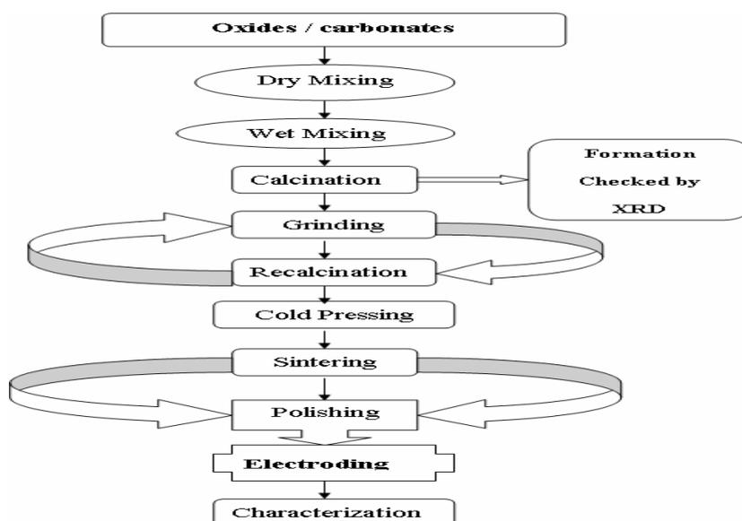
Fig. 2 Flow chart of the mixed oxide route for making PZT ceramics.
