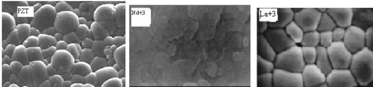
Fig.6. SEM pictures of chemically etched (a) undoped, (b) Nd<sup>3+</sup> doped, (c) La<sup>3+</sup> doped PZT calcined pellets.
