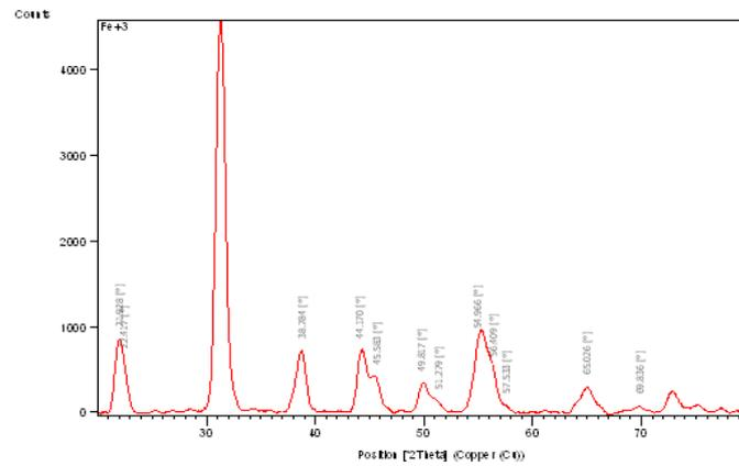
Fig.4. X-ray powder diffraction pattern for the system PbNd (Zr<sub>0.52</sub>Ti<sub>0.48</sub>) O<sub>3</sub>.
