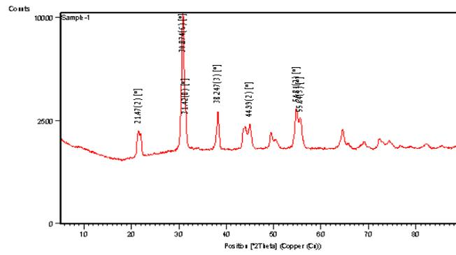
Fig.3. X-ray powder diffraction pattern for the system Pb (Zr<sub>0.52</sub>Ti<sub>0.48</sub>) O<sub>3</sub>.
