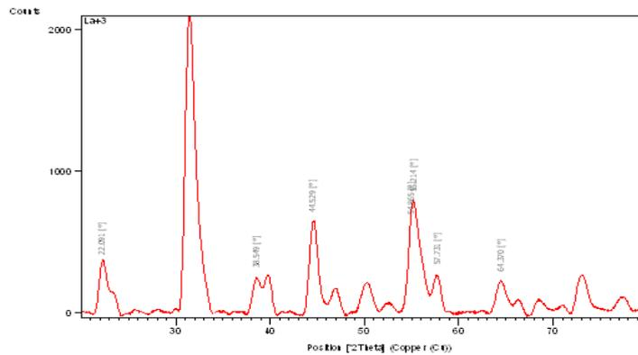
Fig.5. X-ray powder diffraction pattern for the system PbLa (Zr<sub>0.52</sub>Ti<sub>0.48</sub>) O<sub>3</sub>.
