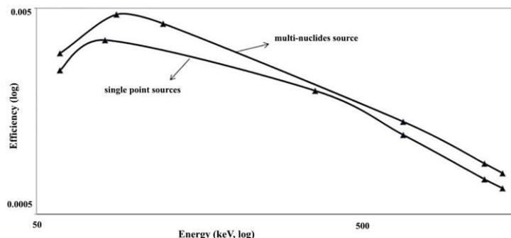
Figure 1. Efficiency versus energy by multi-nuclides source and single point sources at 15.8 cm source-detector distance
