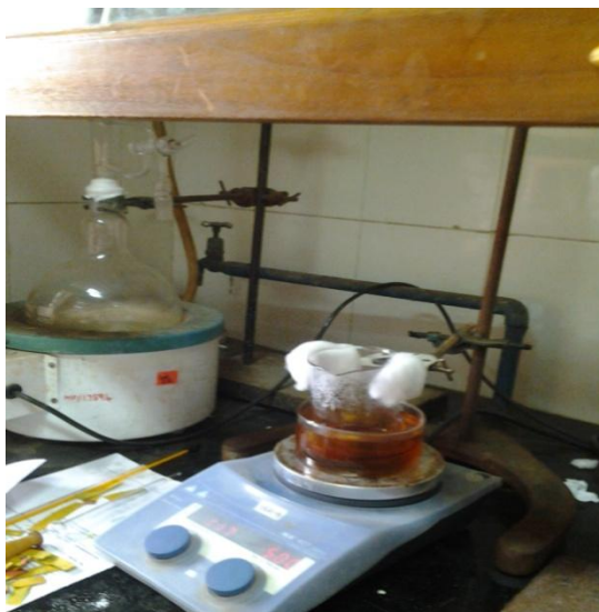
Fig 2. Oil bath & magnetic stirrer cum heater, with precise temperature control and provision for monitoring the number of revolutions per minute .The outer trough contains the oil where the heat energy is distributed equally maintained to the inner beaker
