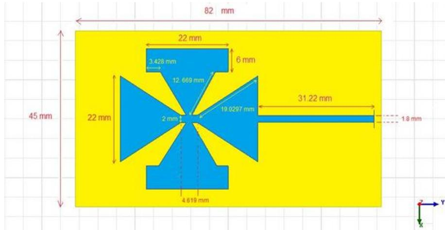
Figure (1): Proposed antenna geometry and dimensions.
