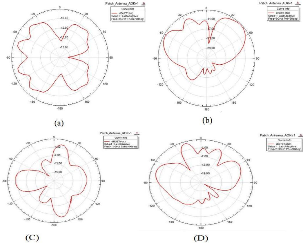
Figure (3):the numerical results of the radiation patterns at different frequencies: (a)  $\theta=90^\circ$  and (b)  $\Phi=90^\circ$  at 9 GHz. (c)  $\theta=90^\circ$  and (d)  $\Phi=90^\circ$  at 11GHz.
