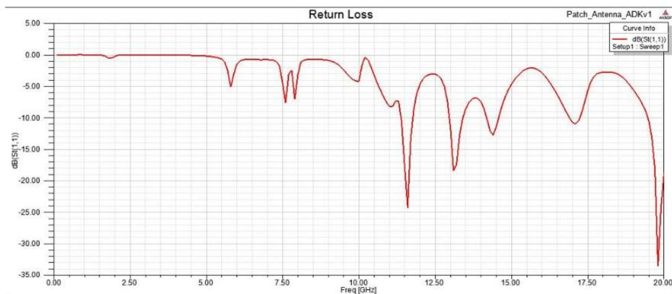
Figure (2) the numerical results,  $S_{11}$ , for the antenna.
