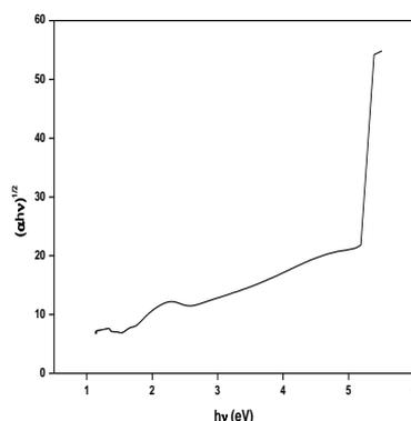
Fig 6. Plot of  $(\alpha h\nu)^{1/2}$  vs photon energy
