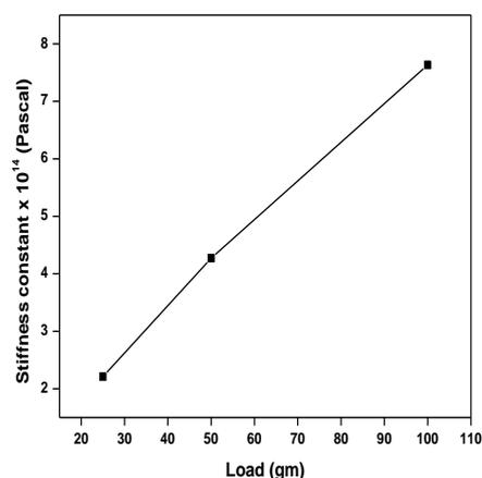
**Fig 11. Variation of stiffness constant with the applied load**
