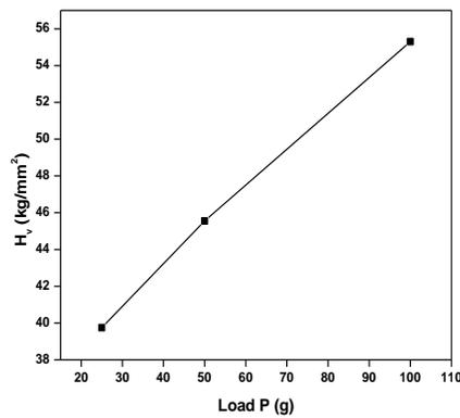
Fig 8. Plot of H<sub>v</sub> vs load P
