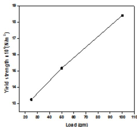
Fig 10. Variation of yield strength with the applied load
