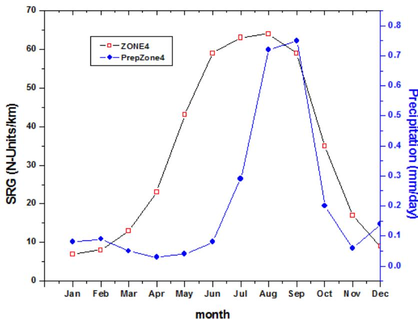
**Figure 6:** Monthly Variation of Surface Refractivity Gradient (SRG) and Precipitation for Climatic Zone 4 in West Africa (1983 – 2005)
