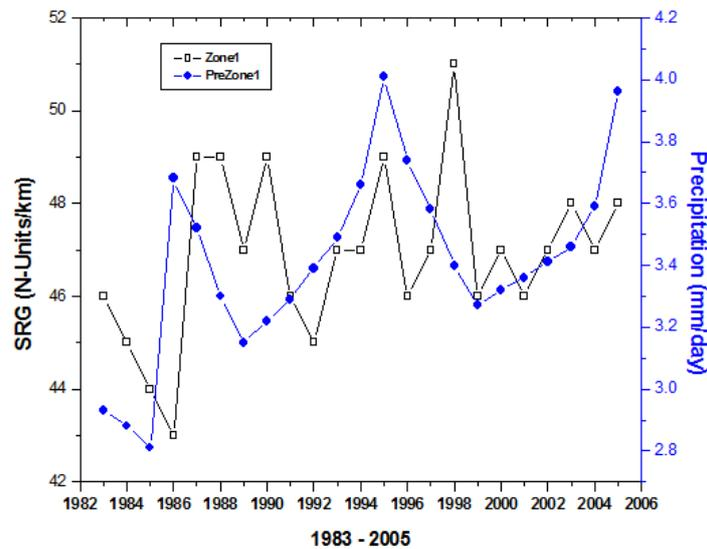
**Figure 7:** Annual Variation of Surface Refractivity Gradient (SRG) and Precipitation for Climatic Zone 1 in West Africa
