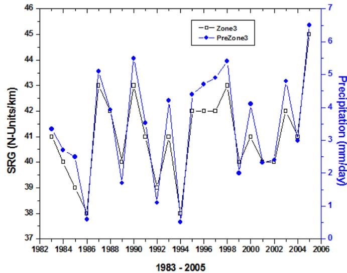
**Figure 9:** Annual Variation of Surface Refractivity Gradient (SRG) and Precipitation for Climatic Zone 3 in West Africa
