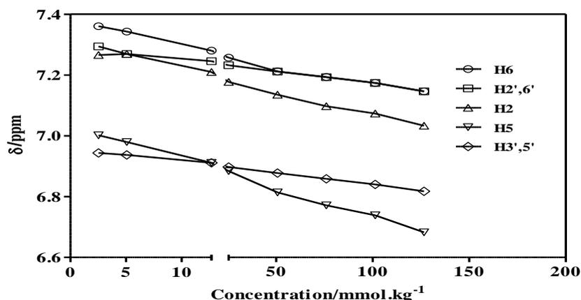
**Figure 6:** Concentration/  $\text{mmol.kg}^{-1}$  vs. chemical shift/ppm of different aromatic protons of itopride HCl in  $\text{D}_2\text{O}$ .
