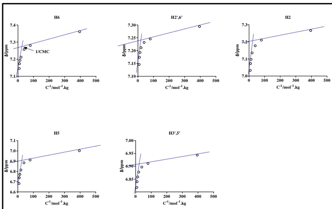
**Figure 5:** Plots of the chemical shift  $\delta/\text{ppm}$  values against reciprocal molal concentration for different aromatic protons of itopride HCl in  $\text{D}_2\text{O}$ .
