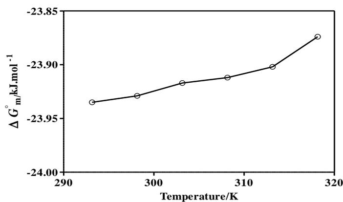
Figure 7: Plots of  $\Delta G_m^\circ/\text{kJ.mol}^{-1}$  vs. temperature/K for itopride HCl aqueous solutions.
