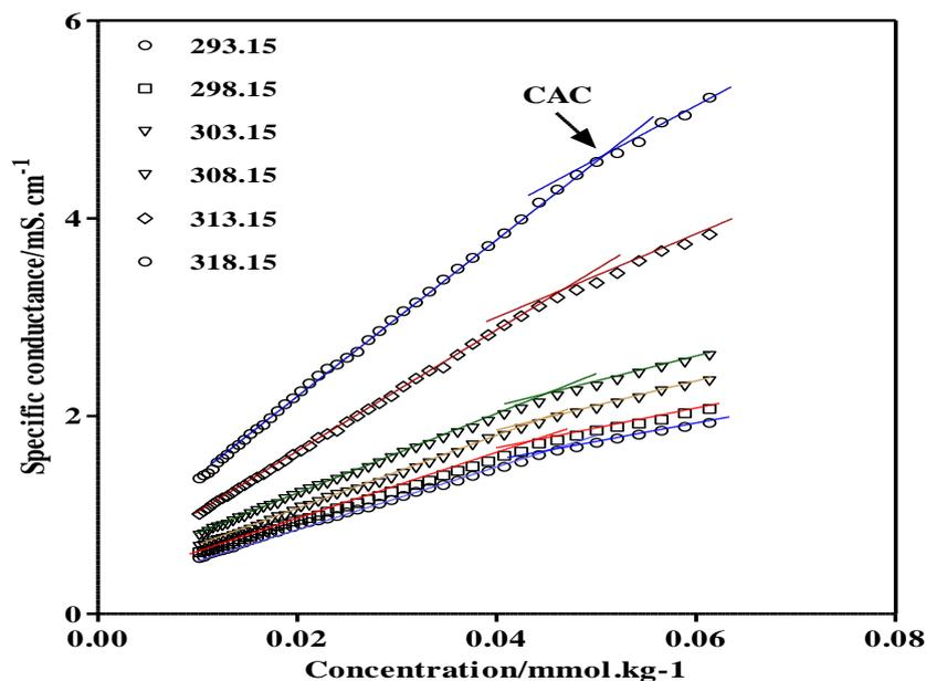
**Figure 1:** Specific conductance/mS.cm<sup>-1</sup> vs. concentration/mmol.kg<sup>-1</sup> plots of itopride HCl aqueous solutions at different temperatures.
