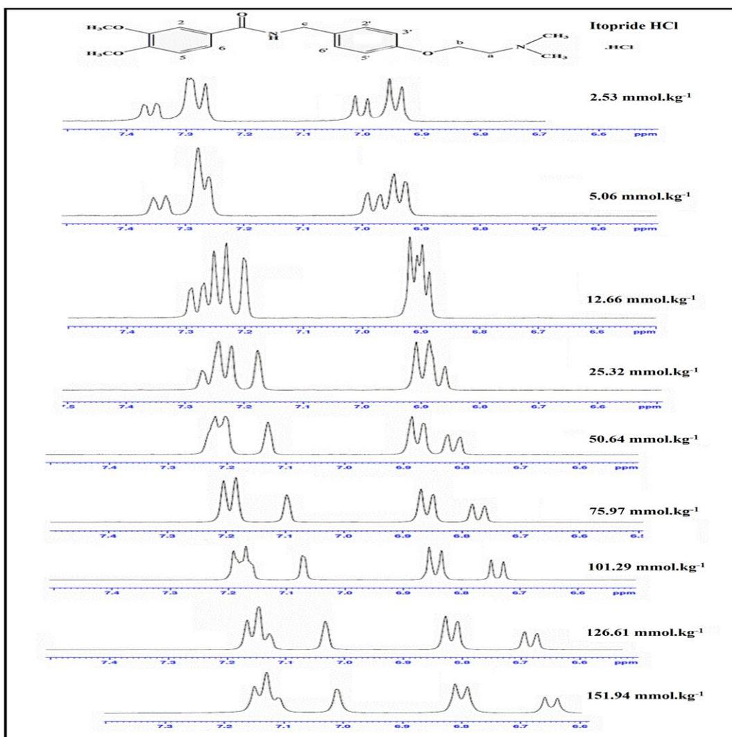
Figure 4:  $^1\text{H}$  NMR of the aromatic protons of different concentrations of itopride HCl in  $\text{D}_2\text{O}$ .
