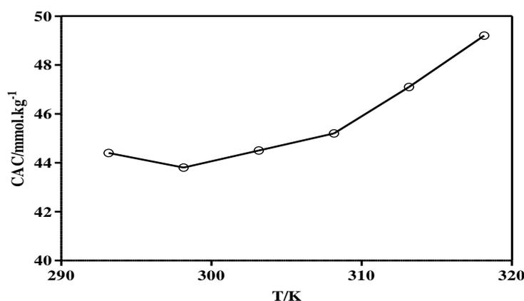
**Figure 2:** Temperature dependence of CAC/(mmol.kg<sup>-1</sup>) of itopride HCl aqueous solutions.
