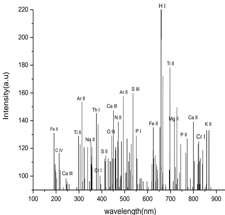
**Figure (2): LIBS emission spectrum of sample (1)**
