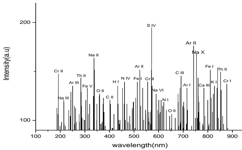
Figure (4): LIBS emission spectrum of sample (3)
