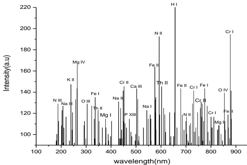
Figure (5): LIBS emission spectrum of sample (4)
