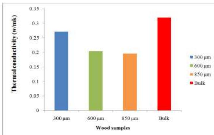
**Figure 1:** Thermal conductivity as a function of wood sample for *Celtis philippensis* (Ita funfun).
