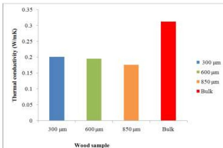
**Figure 2:** Thermal conductivity as a function of wood sample for *Melicia excelsa* (Iroko).
