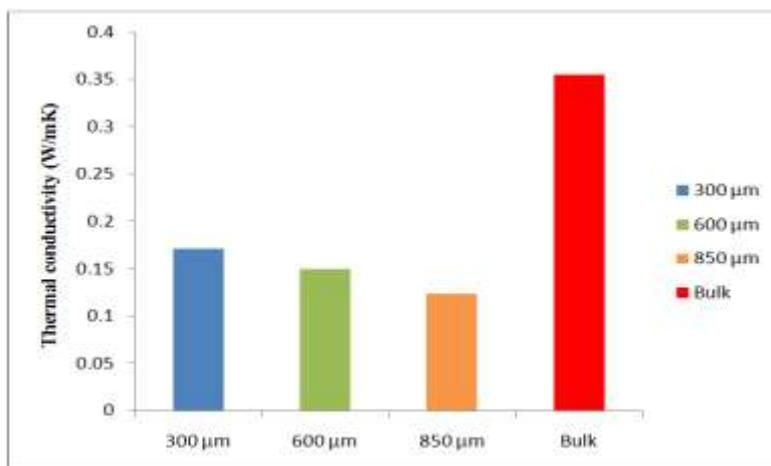
**Figure 3:** Thermal conductivity as a function of wood sample for *Pterygota macrocarpa* (Oporoporo).
