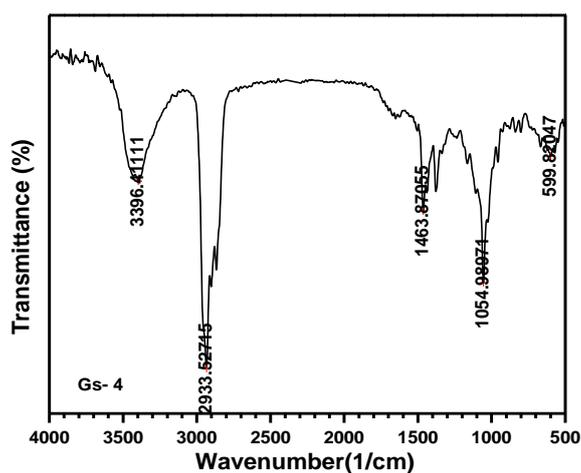
Figure – 3.4: FTIR Spectrum of GS 4
