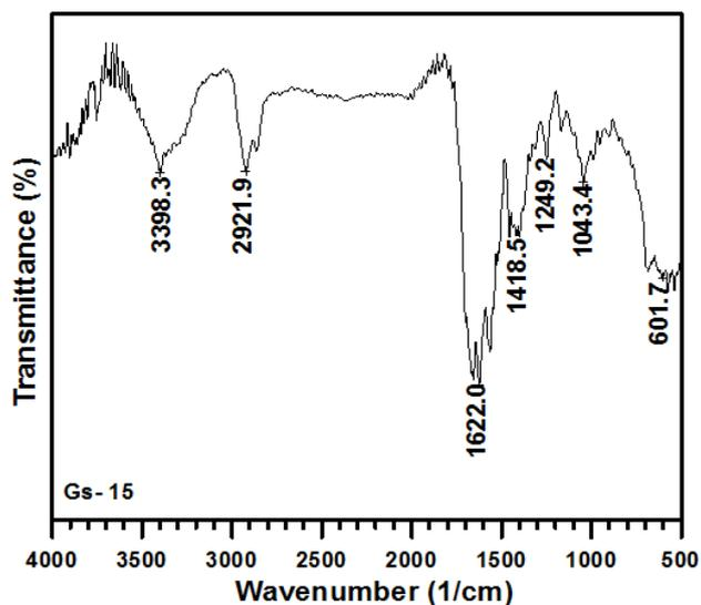
Figure – 3.15: FTIR Spectrum of GS 15
