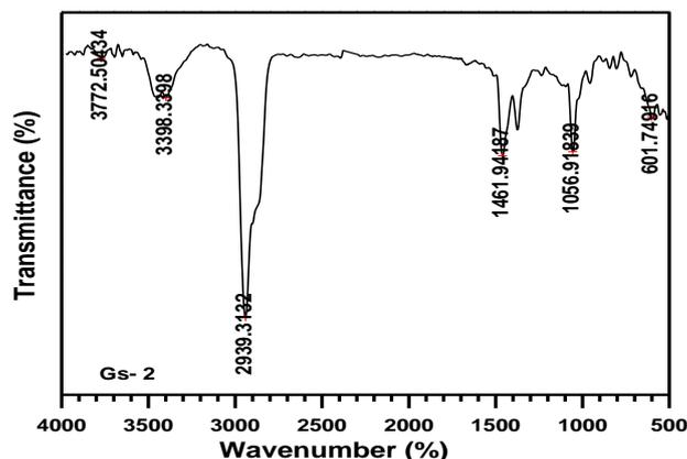
Figure – 3.2: FTIR Spectrum of GS 2
