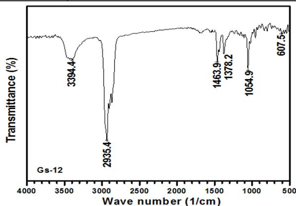
Figure – 3.12: FTIR Spectrum of GS 12
