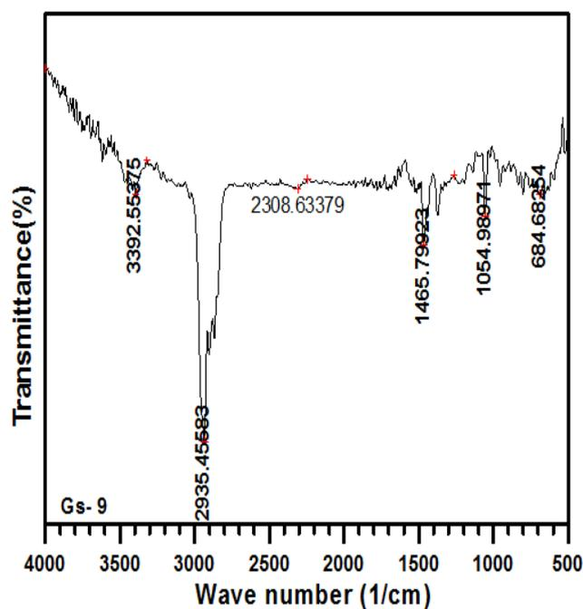
Figure – 3.9: FTIR Spectrum of GS 9
