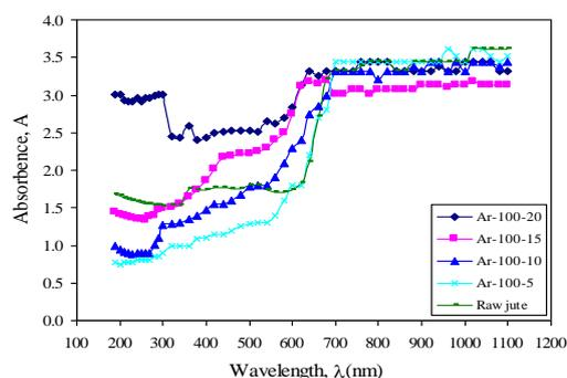
Figure 3 Absorbance vs. wavelength curves for Ar plasma at 100 W
