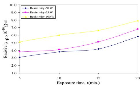
Figure 9 Resistivity vs. exposure time for Ar plasma at different discharge power.
