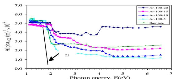
Figure 4 Absorption Coefficient Vs. Photon energy curves for Ar plasma at 100 W (An example of determining of band gap is shown in the case of raw jute fibre)
