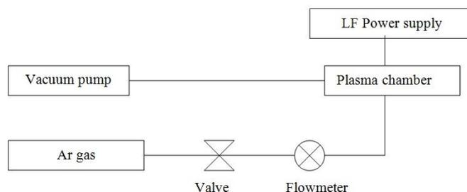
Figure 1. A schematic diagram of the plasma treatment set-up.
