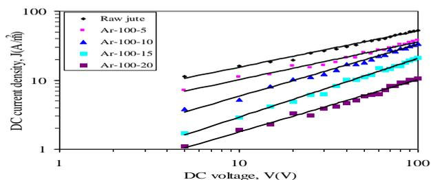
Figure 7 J–V plots for raw and treated jute for Ar plasma at different time at 100 W
