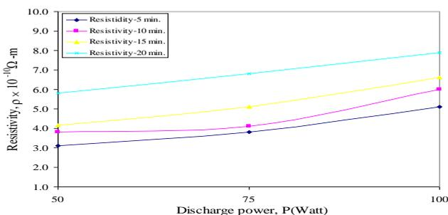
Figure 10 Resistivity vs. discharge power for Ar plasma at different exposure time.
