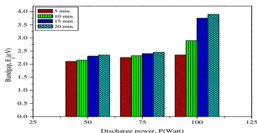
Figure 6 Optical band gap vs. discharge power at different time of Ar gas
