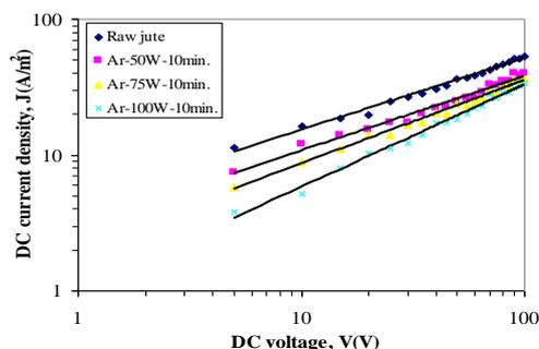
Figure 8 J–V plots for raw and treated jute for Ar plasma with different power at 10 min.
