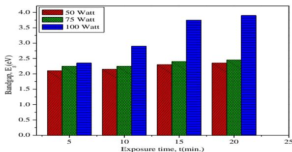
Figure 5 Optical band gap vs. exposure time at different power of Ar gas
