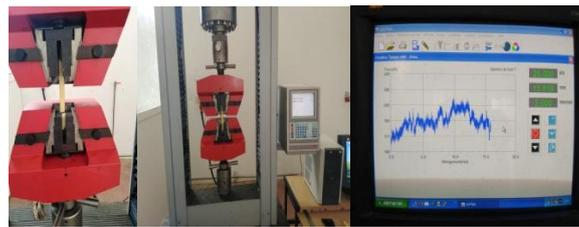
Figure 7: Fixation of the specimen and course of the tensile test
