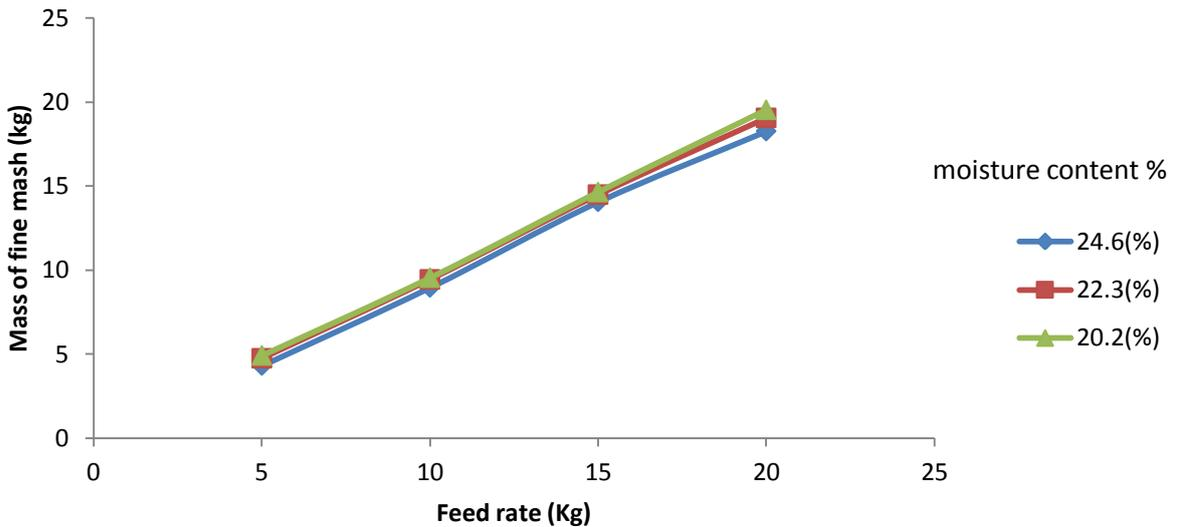
Figure 2: Effect of moisture content and feed rate at 970 rpm
