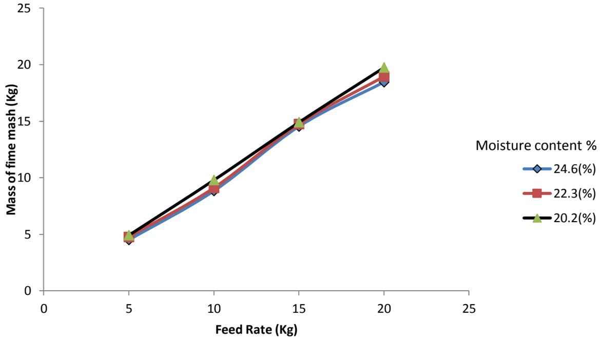
Figure 1: Effect of moisture content and feed rate at 1200 rpm
