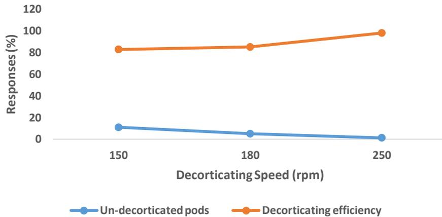
Figure 6: Evaluation at 5 kg Peanut Kernel quantity and decorticator efficiency
