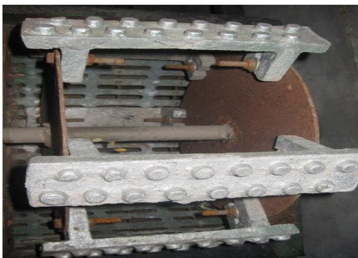
**Figure 2: Screen and decorticating drum of the decorticator**
