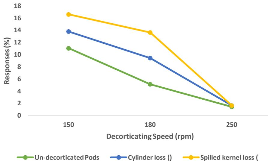
Figure 7: Evaluation Losses at 5 kg Peanut Kernel quantity
