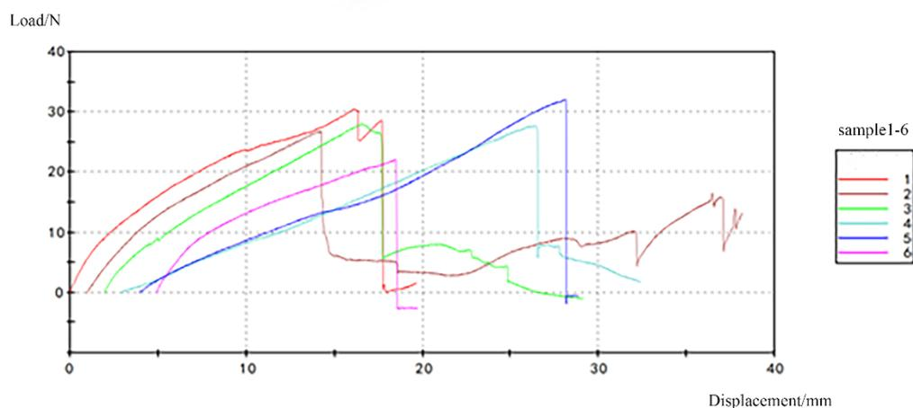
Figure 3. Tensile load of Root
