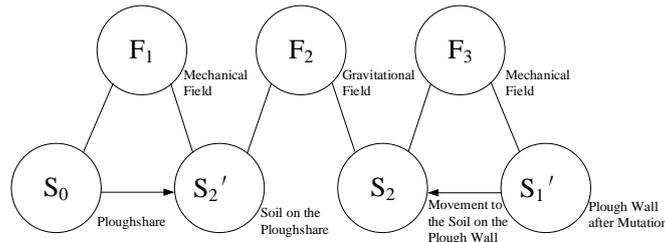
Figure no 3 : Complete object-field model of the main plow body.
