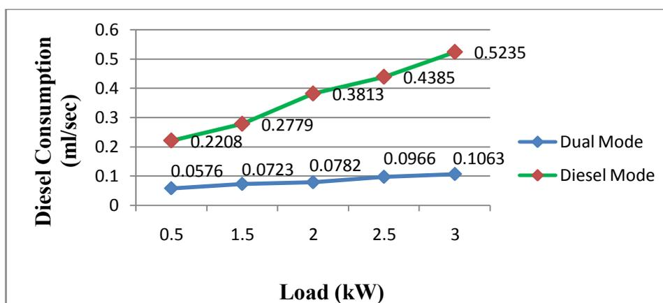
**Fig. 3.14 Diesel Consumption v/s Load Dual Mode of Engine (Cotton Stalk)**
