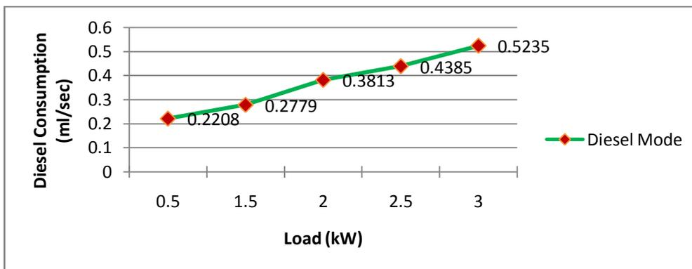
**Fig. 3.13 Diesel Consumption v/s Load in Diesel Mode of Engine**
