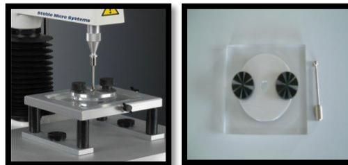
**The 5 mm stainless steel spherical probe (P/5S) and Perspex film support platform with Aluminum circular top plate used in Texture analyzer.**
