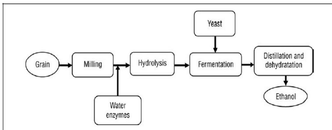
Fig 1. Ethanol production from grain dry milling (Reith et. al, 2001)
