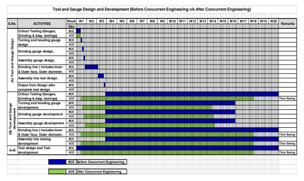
Figure 3. Tools and Gauges design and development
