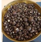
Figure 1 shows the completed sintering process, which represents the closing of pores associated with the mechanical strength of the aggregates. The efficiency of solid-state reactions is responsible for the formation of mullite and the vitreous phase. These interactions can be controlled through adjustments in the granulometry of raw materials, sintering temperature and time, and matrix formulation<sup>14,15</sup>.
