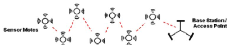
Fig.1 MESH topology of sensor nodes
