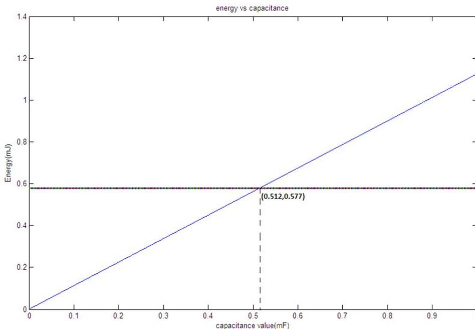
So it is possible to use Broad Sensor Network using given circuit of super capacitor having capacitance value approximately equals to 0.512mF
