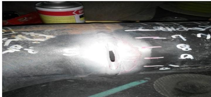
Figure 1: A pipeline showing Crack with measurement (picture courtesy-SADARA,KSA)
