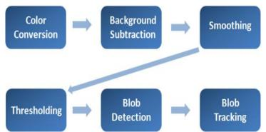
Fig.8 Image Processing Steps for extraction, detection and tracking of the blobs.
