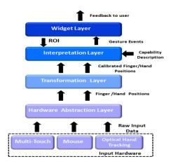
Fig. 7 Multi-Touch Sensing Software Architecture
