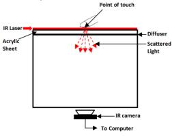
Fig. 5 Setup for LLP
