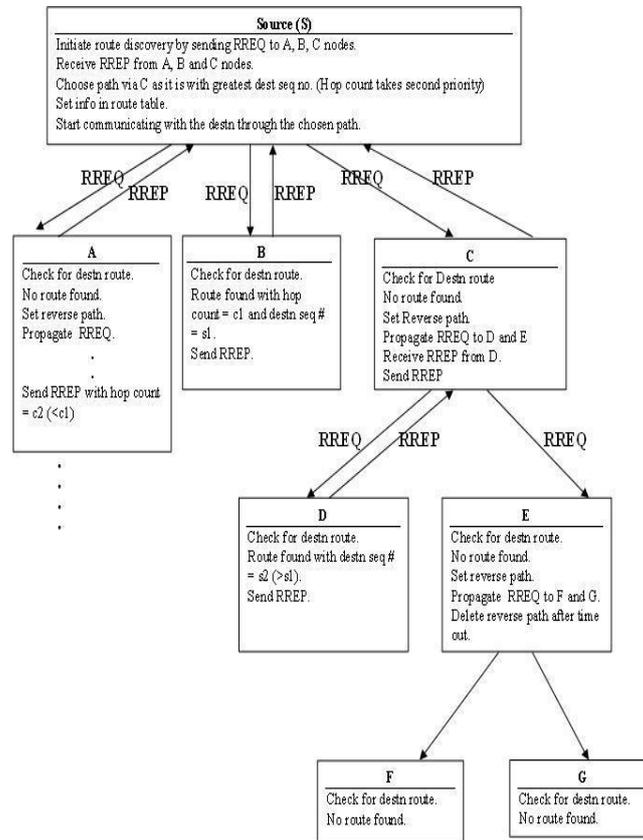
Fig. 3. Architecture of Complete System
