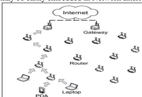
Fig. 2. A typical wireless mesh network
