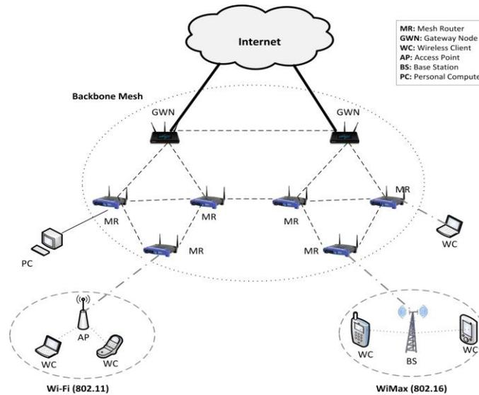
Fig. 1. Typical Wireless Mesh Network Architecture
