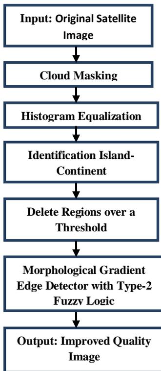
Fig.3. Image processing module
