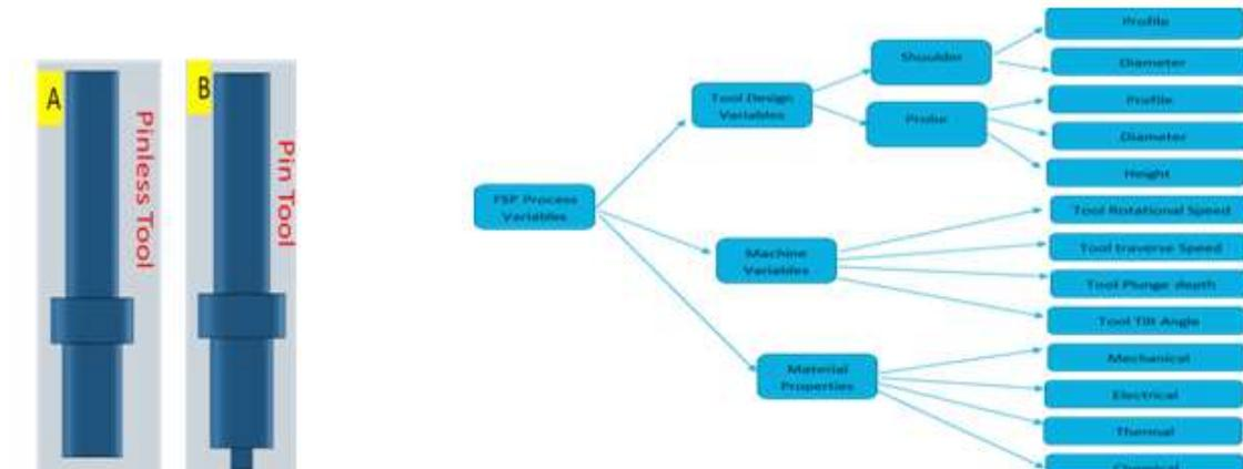
Figure 3: FSP Tool (a) For Compaction (b) For Stirring Figure 4: Flowchart of Process Variables used in FSP
