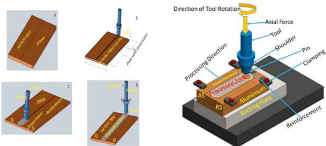
Figure 1: Schematic of a typical FSP Figure 2: Schematic of FSP showing Advancing and Retreating Side
