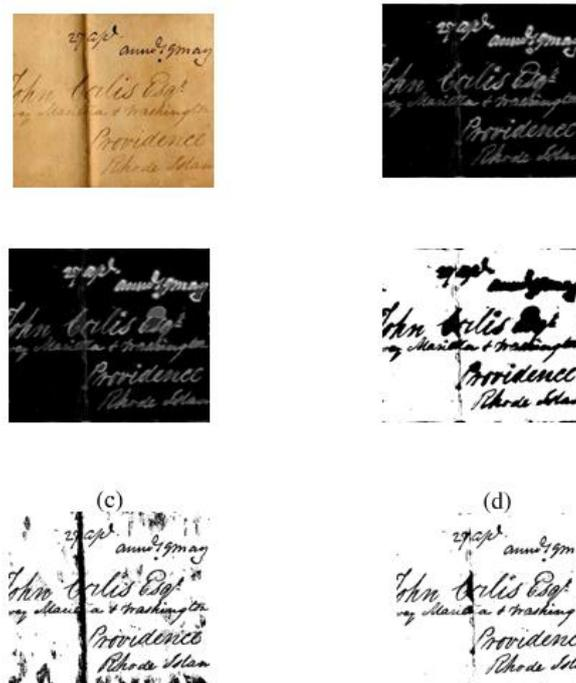
Fig. 4. A degraded document image and its binarized image using phase congruency. a) Original degraded document image. b) Edge image obtained by phase congruency ( $IM$ ). c) Filled image of  $IM$ . d) Binarization of (c) using Otsu’s method. e) Denoised image and f) The result of main binarization.
