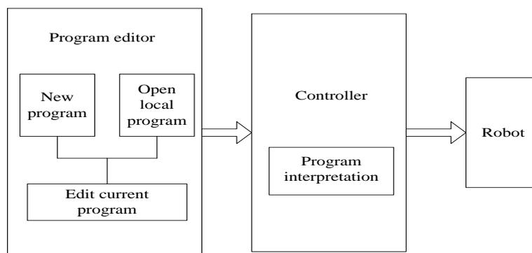
Fig.5 Program editing function realization process
