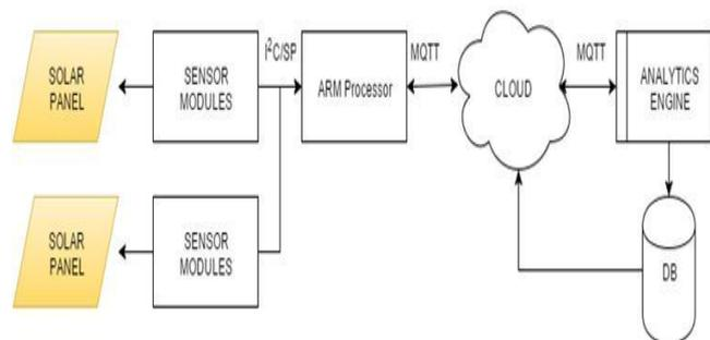
**Figure 1:** Data Acquisition Architecture
