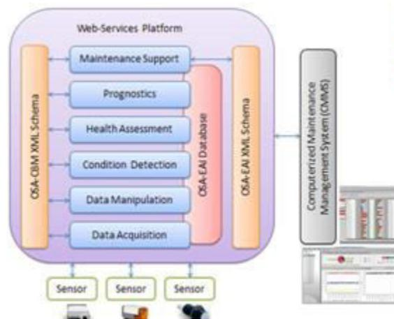
**Figure 4. Reference architecture for condition-based maintenance mgmt. system**
