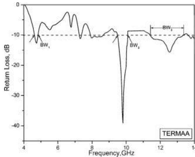
Figure 4 Variation of return loss versus frequency of TERMAA
