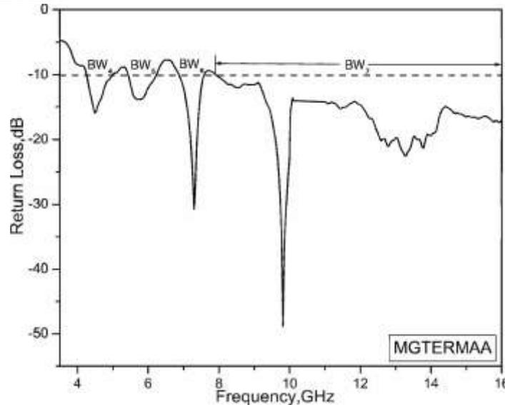
Figure 5 Variation of return loss versus frequency of MGTERMAA
