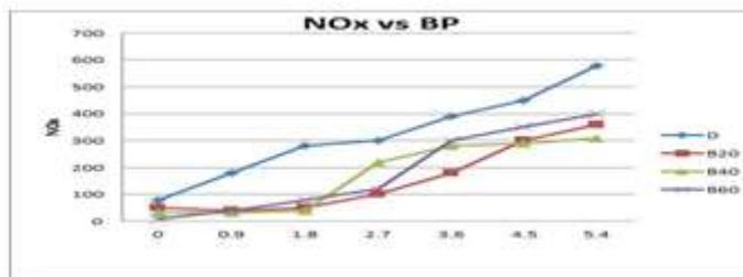
**Figure 3** Nox VS Break Power
