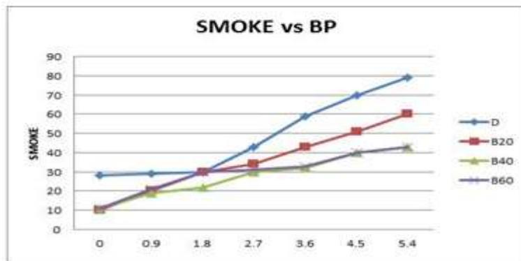
**Figure 6** Smoke vs Break power
