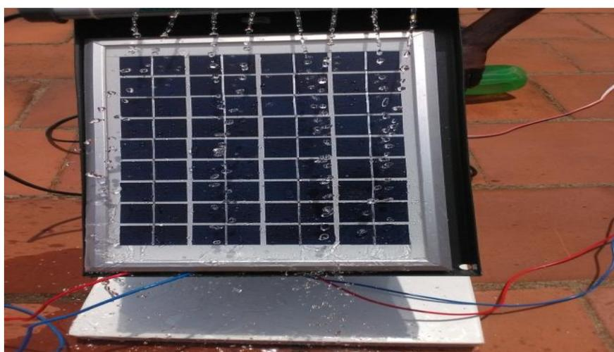
**Fig 3.5 automated water spraying on solar panel**
