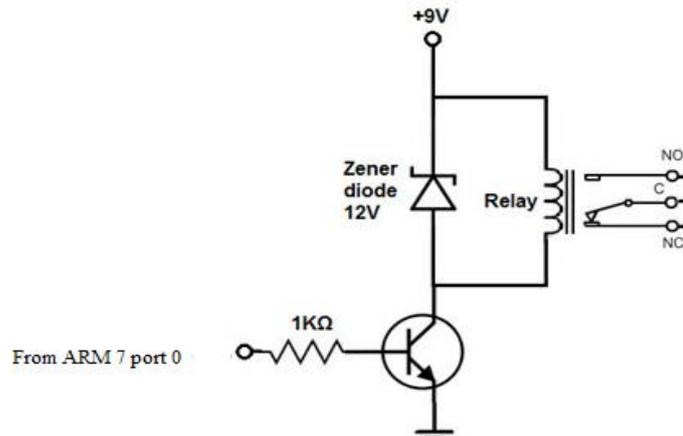
Fig 2.3 Relay Driver Circuit
