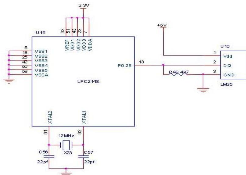
Fig 3.2 Signal Conditioning Unit With LM 35
