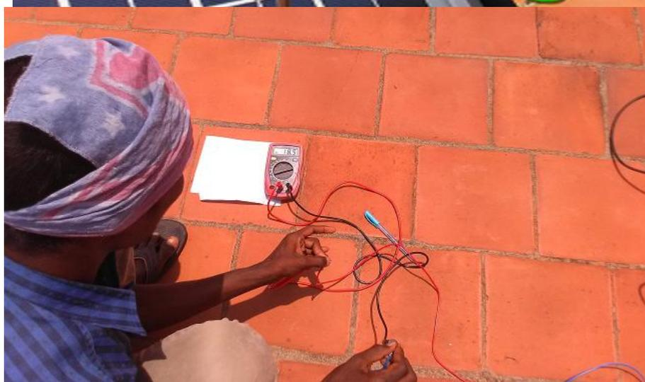
**Fig 3.4 At 12.30 hours panel temperature and panel voltage measurement**
