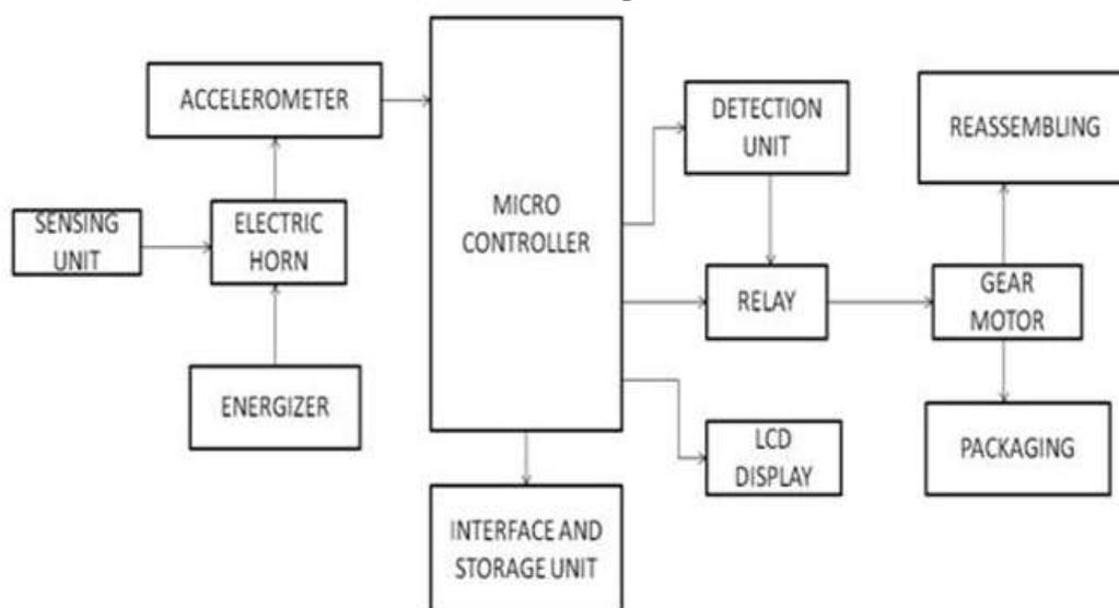
Figure 1 Block Diagram
