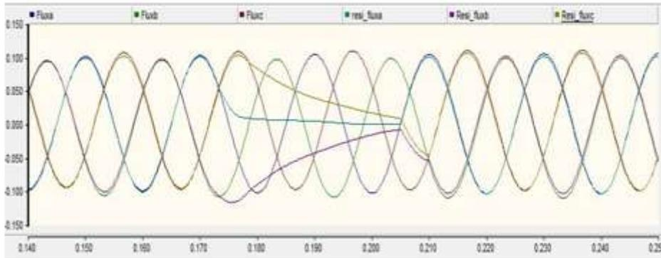
Figure 9 Prospective Flux and Residual Flux (Ideal Case)
