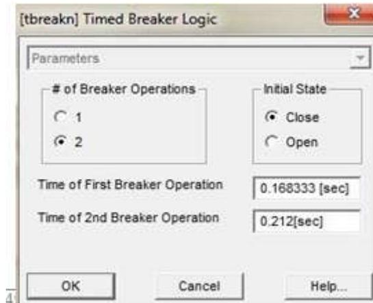
Figure 16 Breaker 3 Logic (Case 1)
