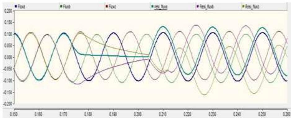
Figure 21 Prospective and Residual Flux (Case 3)
