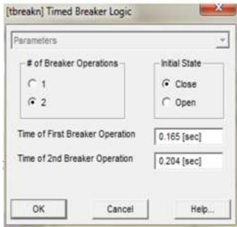
Figure 22 Breaker 1 Logic (Case 3)..
