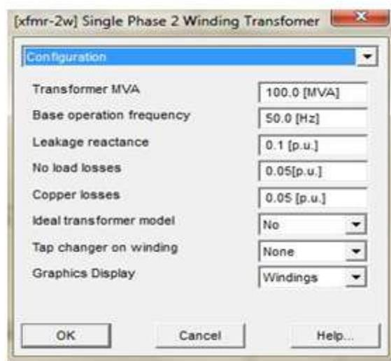
Figure 7 Configuration of Transformer
