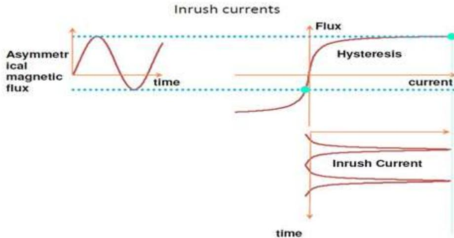
Figure 2 Transient flux
