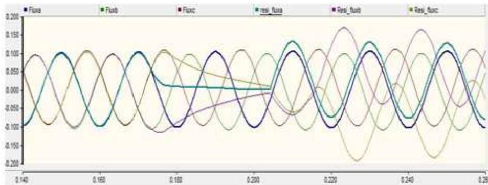
Figure 17 Prospective and Residual Flux (Case 2)
