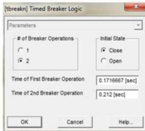
**Figure 15** Breaker 2 Logic (Case 2)
