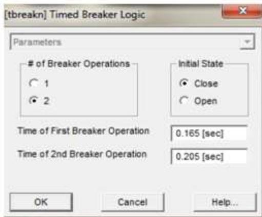
**Figure 14** Breaker 1 Logic (Case 1)
