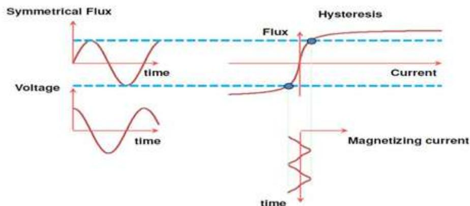
Figure 1 Magnetic flux in steady state
