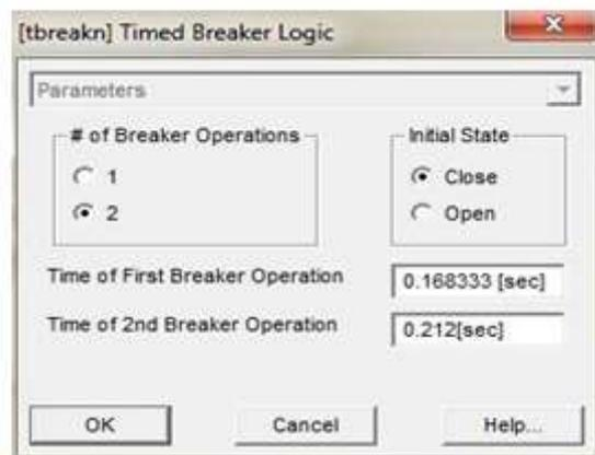
Figure 24 Breaker 3 Logic (Case 3)
