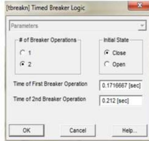
Figure 23 Breaker 2 Logic (Case 3)
