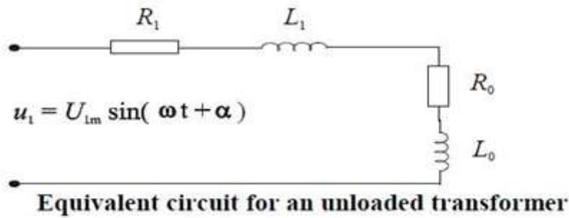
**Figure 4** Equivalent Circuit for an unloaded transformer (Reference: Damascus Univ. Journal
