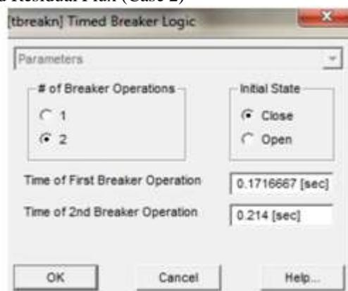
Figure 19 Breaker 2 Logic (Case 2)
