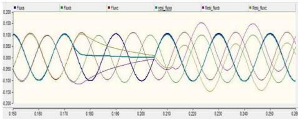
**Figure 13** Prospective Flux and Residual Flux (Case 1)
