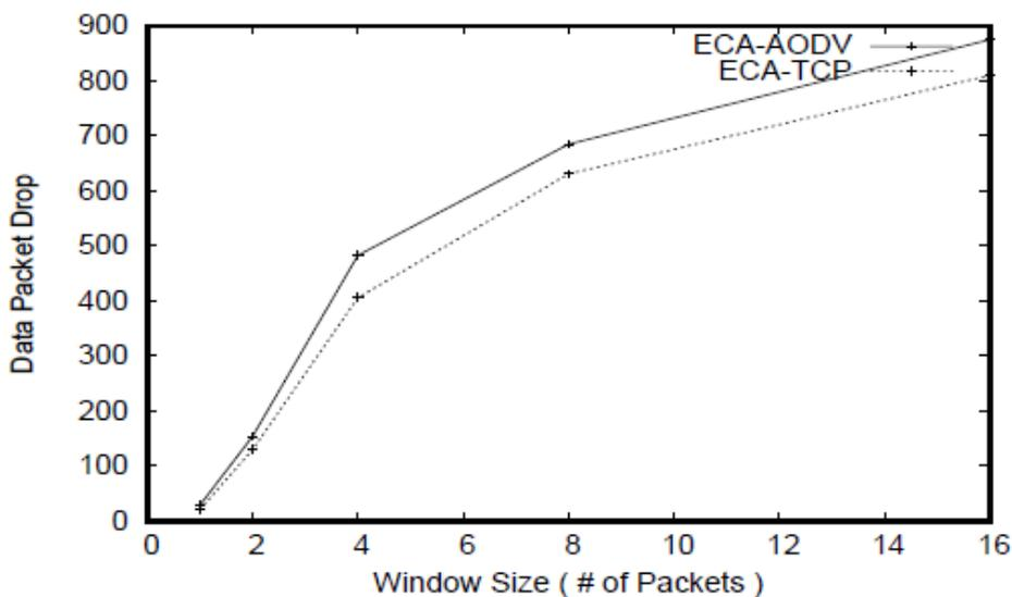
Fig. 10: Effect of Packet Drop Due to Window Size
