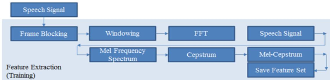
Figure 2 Block diagram of MFCC Feature extraction
