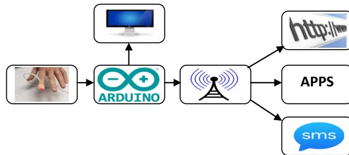
Figure no 11: System Model for Oximeter Sensor
