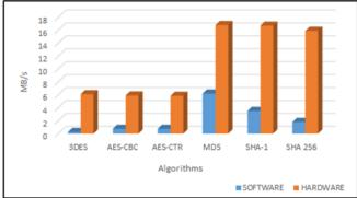
Fig.1Efficiency of Various Hashing Algorithms
