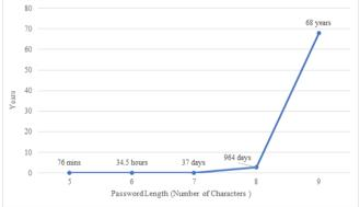
Fig.6Attack Complexity Analysis of Anti-password Algorithm
