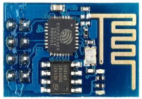
Fig. 2. ESP8266 Serial WiFI Module (ESP-01)
