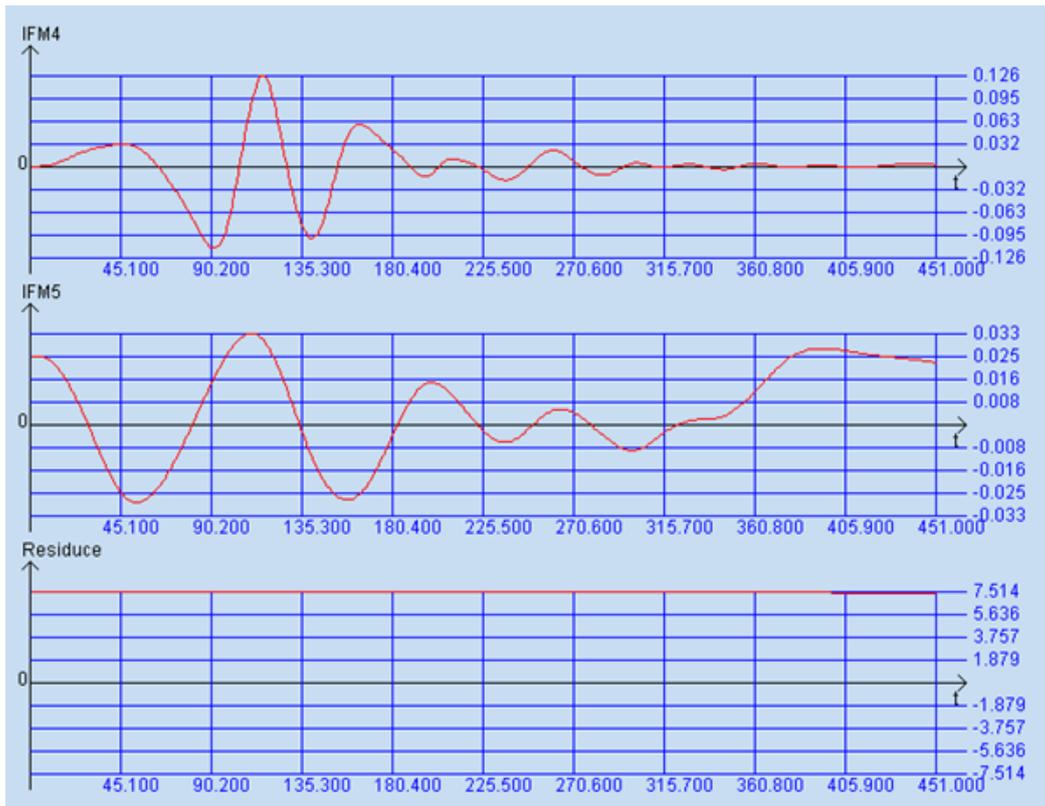
**Figure 8.** The IMFs of PH signal.
