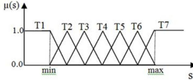
**Figure 5.** Membership function for input and output.
