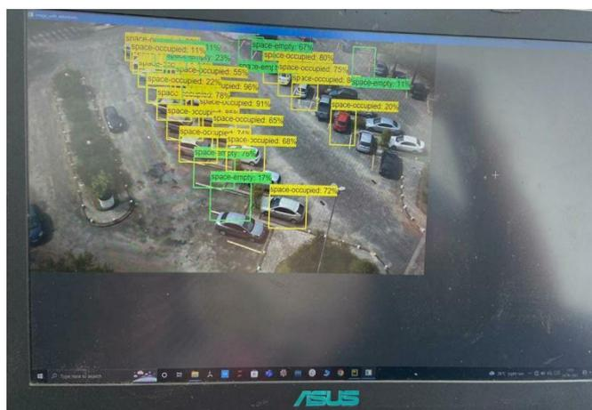
Following the training, the inference graph was exported. The classifier used for object detection is contained in the inference graph. Figure depicts the sample detection with cars parked in a parking lot. Some cars and empty parking lots were not recognised by the SSD using ResNet. Even though this model has some loss, real-time applications can use its fast detection.
