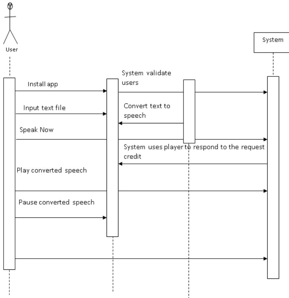
**Figure 2: Sequence Diagram of the Proposed System**
