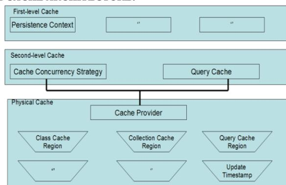
Figure 2 : Two-level cache architecture
