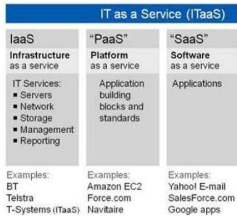
Fig. 3 Three types of Cloud service models
