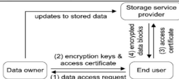
Figure 2. Illustration of application scenario
