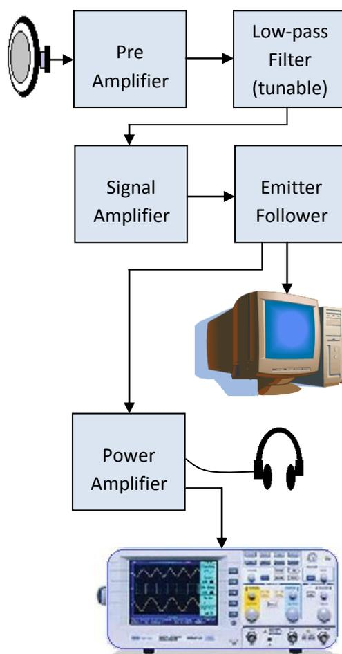
Figure 1: Block diagram of the proposed PCG machine
